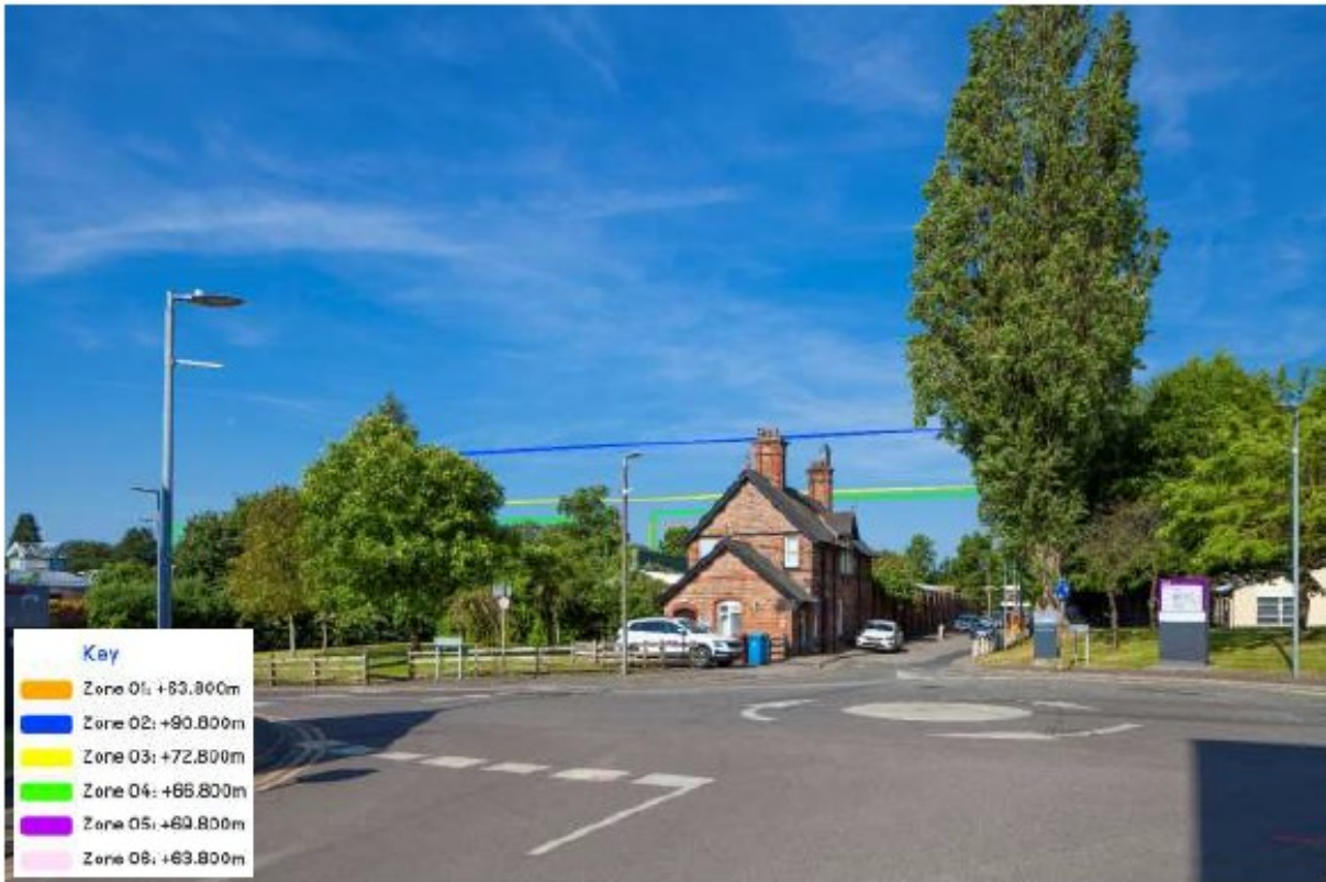
Wireline diagram showing respective heights of proposed buildings set out in the parameters plan view from Gunner Lane looking west towards the application site
